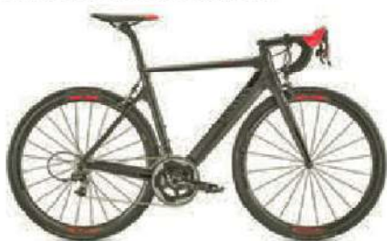
Canyon Aeroad CF 9.0 SL 4299 € Cadre: monocoque carbone – Transmission: Sram Red – Roues: Reynolds Assault – Poids: 6,75 kg
