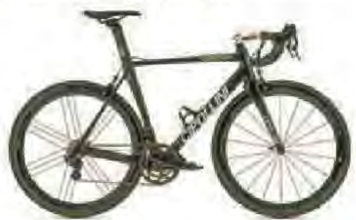
Cipollini RB800 12 671 € Cadre: monocoque carbone – Transmission: Campagnolo Super Record EPS – Roues: Campagnolo Bora Ultra – Poids: 7 kg
