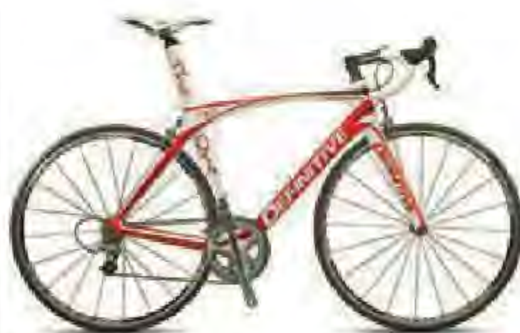
Definitive The One 1999 € Cadre: carbone monocoque – Transmission: Shimano Ultegra – Roues: Mavic Equipe – Poids: 7,9 kg
